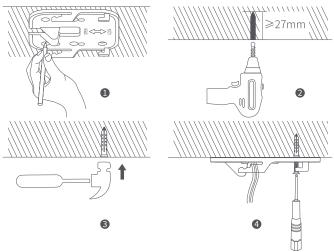
Align the bracket hole at the bottom of the device with the bracket buckle, and push the product body in the opposite direction of the bracket hooks until it is buckled tight (make sure the power cable or Ethernet cable is properly connected before it is tightened).
