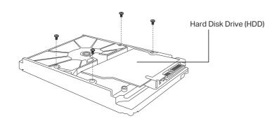
3. Match the 4 screws on the HDD with the 4 holes on the NVR, and insert the HDD interface into the slot.
