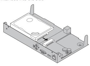
4. Flip the NVR upside down and fasten the HDD screws. Replace the cover and fasten the screws of the NVR.
