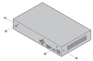
2. Attach the 4 included HDD screws to your hard drive. Do not fasten.
